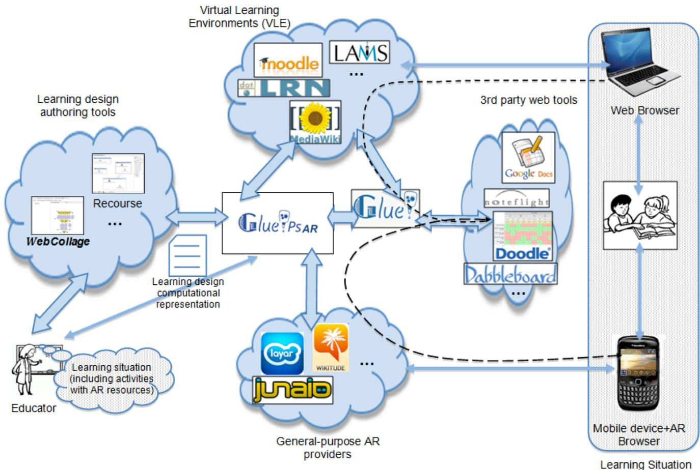
Fig. 1. General architecture of the GLUE!-PS AR proposal
